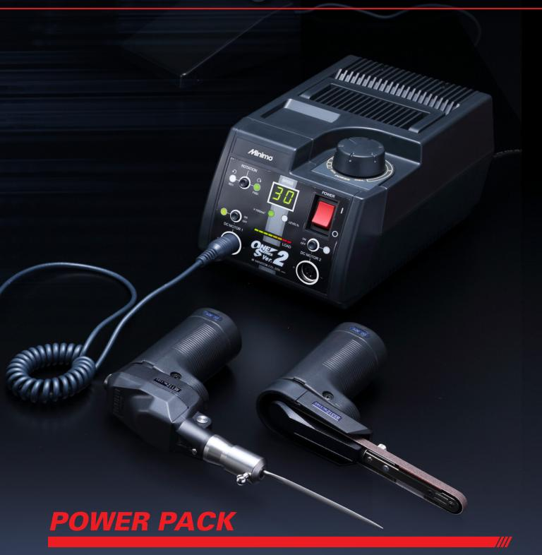
The high-end power pack mounts new functions which maximize the performance of Minitor hand-pieces. This power pack identifies the type of the connected handpiece, displays rotation speed, and controls optimum torque. It is also compatible with the earlier handpieces which do not have the motor identification chip, and gives you more powerful feeling with digital display of its output rate (%).
