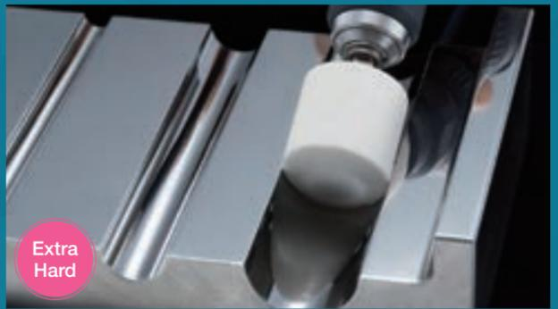
Enable to provide more precise lapping by tight fitting on surface due to retaining felt shape.
