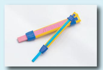
Holder for 3 different size abrasive stone sticks:  $3 \times 6$ ,  $3 \times 13$  and  $6 \times 13$  mm.
