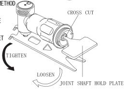
ATTN: WHEN LOOSENING AND TIGHTENING THE COLLET CHUCK WITH THE V-SPANNER. ALWAYS PLACE THE TEST ROD IN THE COLLET CHUCK TO PROTECT THE COLLET FROM TWISTED OR BROKEN.
