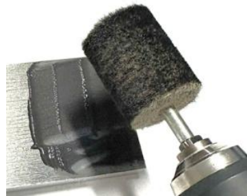
Lubricant-Impregnated Structure. The lubricant is released during operation to suppress heat generation while polishing.
